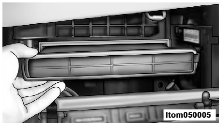
Fresh Air Filter Location
